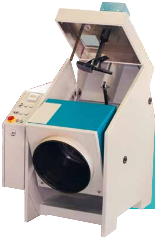
Mixing drum tilted to empty mix
